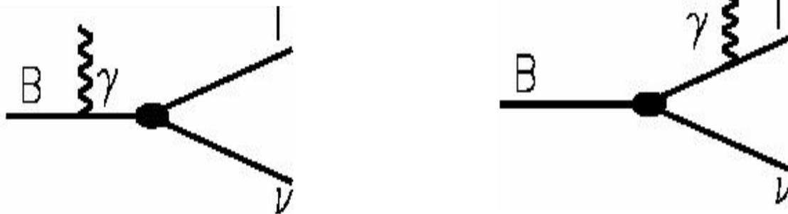
$$M_{IB} = ie \frac{G_F}{\sqrt{2}} V_{ub} f_B m_l \epsilon_\mu^* L^\mu$$
