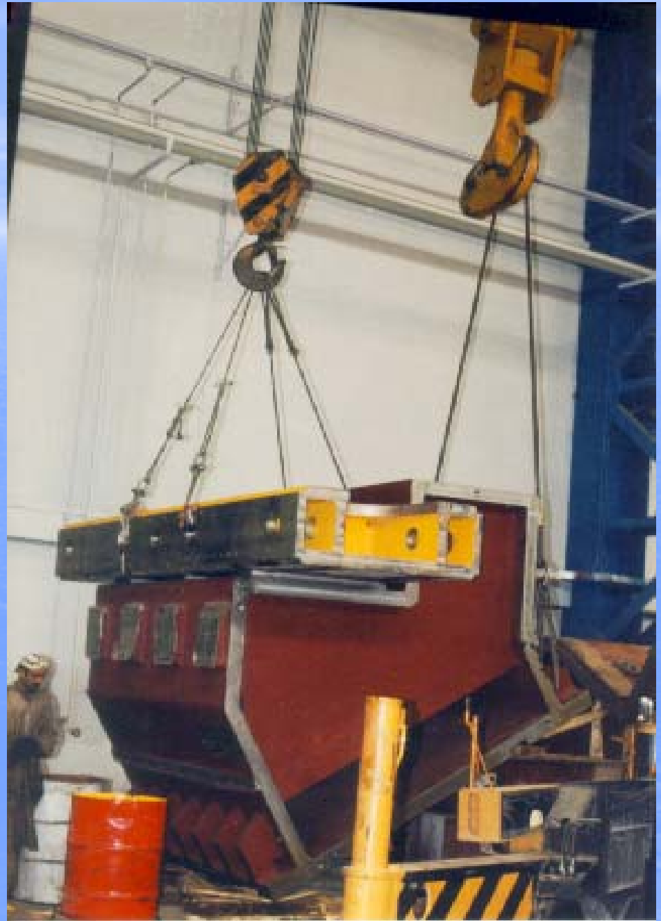
Magnet Support (28.5 Tons)& Transport Beam (10.5 Ton)
