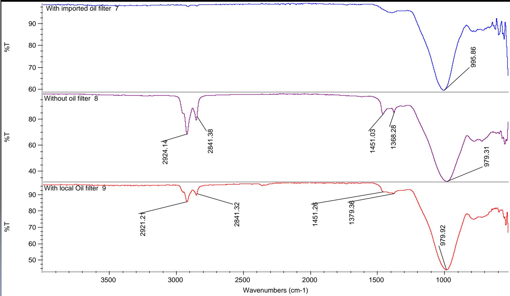
The FTIR spectra of samples with imported, local made and with out OME using Canopus oil in vacuum pump.
