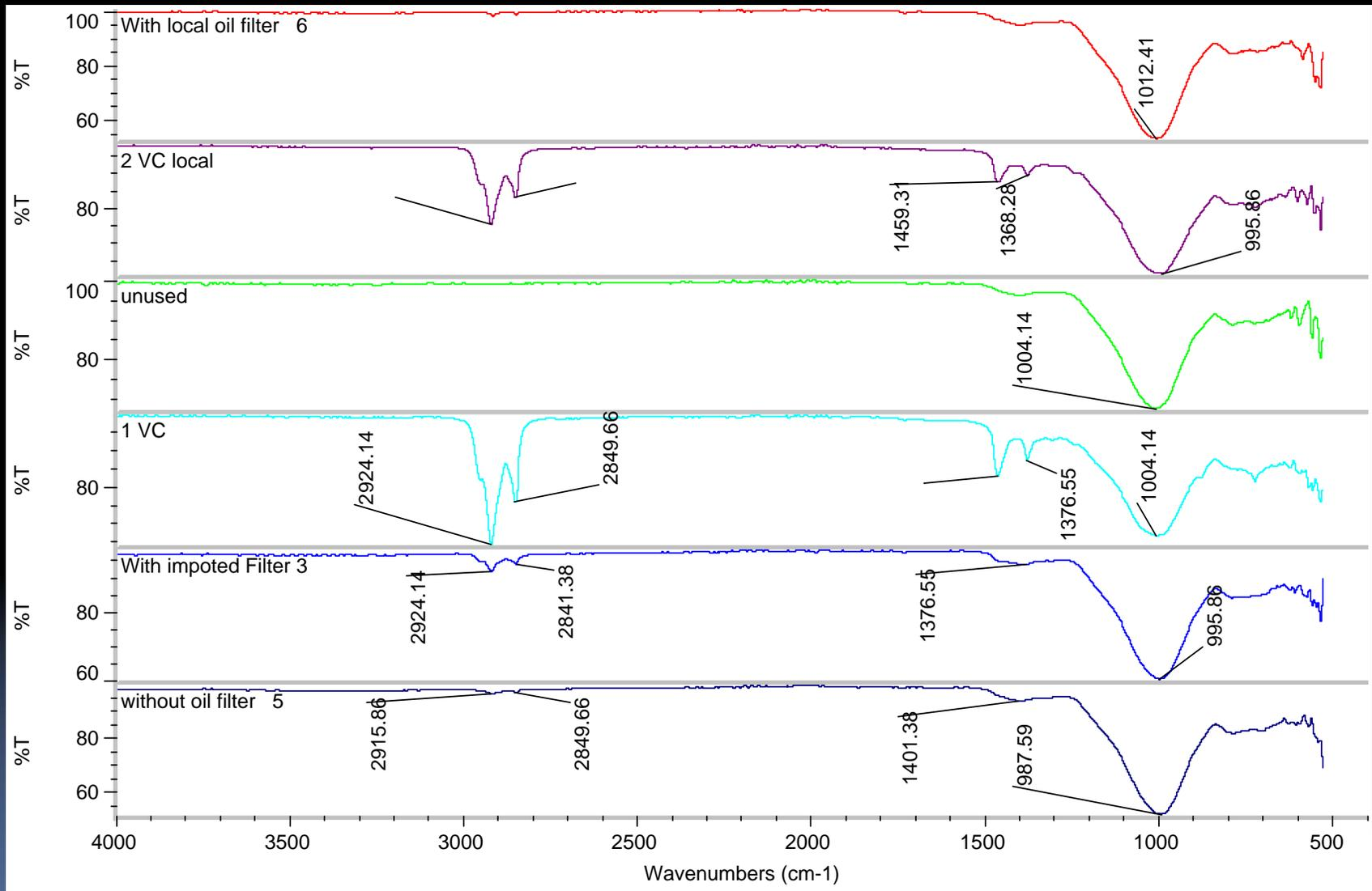
**Comparative FTIR spectra of samples without, with imported, with local made OME and of unused test paper using M 100V oil in the vacuum pump.**
