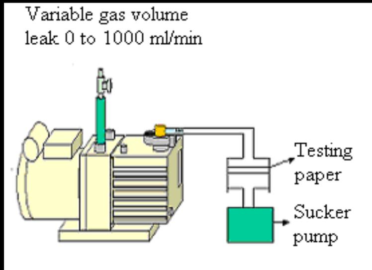
Vacuum pump exhaust sample collection without OME.
