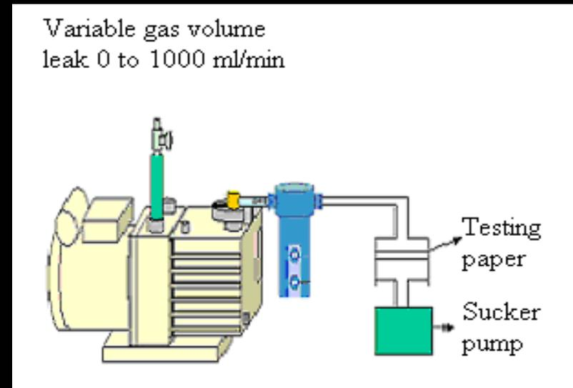
Vacuum pump exhaust sample collection with OME.
